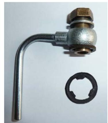
breather pipes allowing the air pressure in the float chamber to remain at atmospheric.
