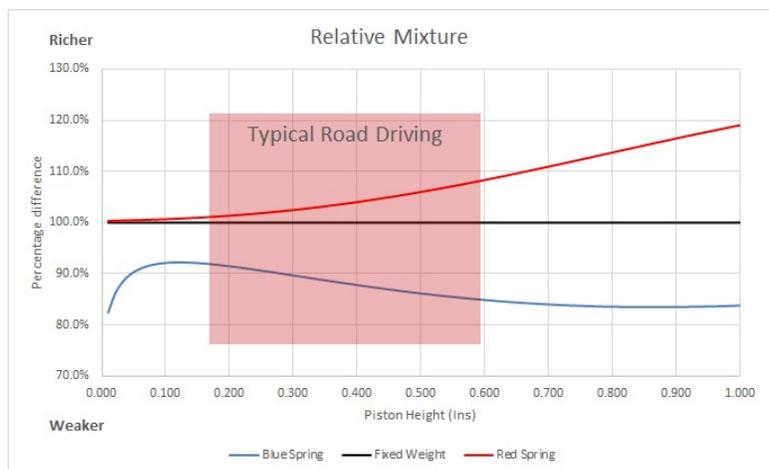
Over the normal range of piston heights used for driving on the road, the ES needle can be used in all three cases. Carburettors fitted with a blue spring can be made richer by screwing out the jet adjusting
