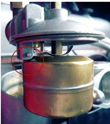
Should you adjust the forks, it's worth inserting a pencil through the hole in the lid and the centre of the float to check it does not foul the pivot support (highlighted on the picture by the red circle) before the needle valve shuts off.
