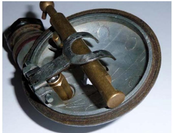
There is a problem. This time not caused by modern petrol! With an HS type of float chamber and the correct fork setting, a float weighing 28gm to 30gm is needed to achieve a fuel level of 3/16" below the jet bridge (approximately half way between 1/8" and 5/16" recommended in the factory handbook for the TC). The original brass floats weigh 24gm which gives a petrol level below the jet bridge of 3/8" (as normally specified for SU carburettors).
