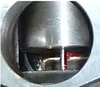
A photograph of the carburettor taken during the first set of tests shows the (artificially coloured red) petrol leaving the jet as a stream rather than a dispersed mist. Something not seen in the second set of tests.
