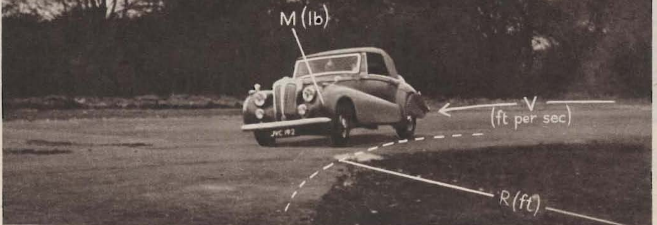
CENTRIFUGAL FORCE. This photograph of a car cornering at speed shows the violent effect of the centrifugal "pushover," as it also illustrates the dimensions used to calculate the force applying.
