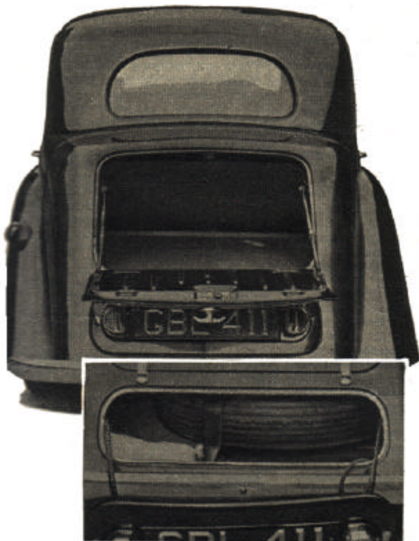
Because the locker lid is hinged at the bottom the useful luggage carrying capacity can be considerably increased by using the lid as a platform. (Inset) A separate lower compartment houses the spare wheels and tools.
