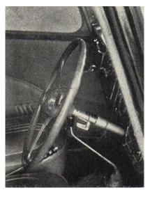
The steering column is adjustable for a 3 in. movement, and the 16in. diameter wheel is spring spoked. Steering is by rack and pinion type gear which is light and positive.
