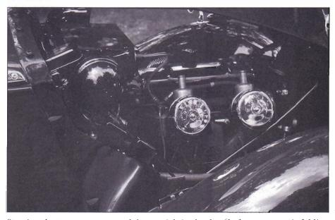
Stowing the top was a pretty elaborate job in the days before automatic folding mechanisms. The engine is original and provides adequate power, but the gearing ratios were changed by using an MGB differential and 15-inch wheels.
