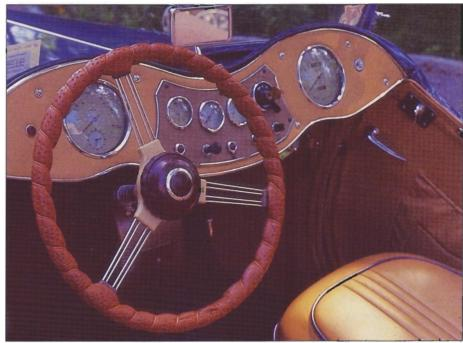
The dash of the Y-Type is the same as the MG-TC but the TC was never available in left-band drive. Like the TC, the windshield folds. Hardware such as door bandles and top clamps is original, and bas been re-chromed. The contrasting upholstery piping is correct; period photos of new cars show it.
