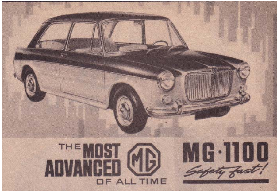
The 1963 MG 1100, with a transverse four-cylinder engine, FWD and front disc brakes
