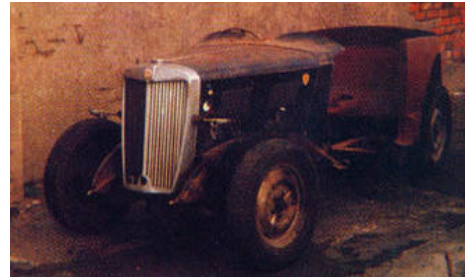
The YT as found – almost all of the bodywork from the rear of the windscreen needed to be rebuilt.
