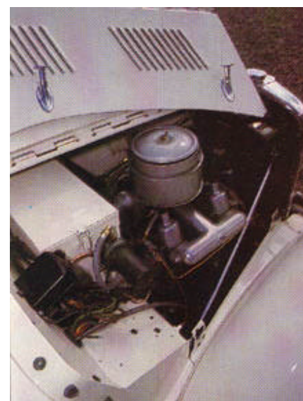
Replacement valves, valve guides and seats were fitted so that the engine could run on unleaded petrol.
