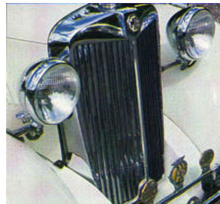
Grille and windscreen surround were rechromed by Derby Plating
