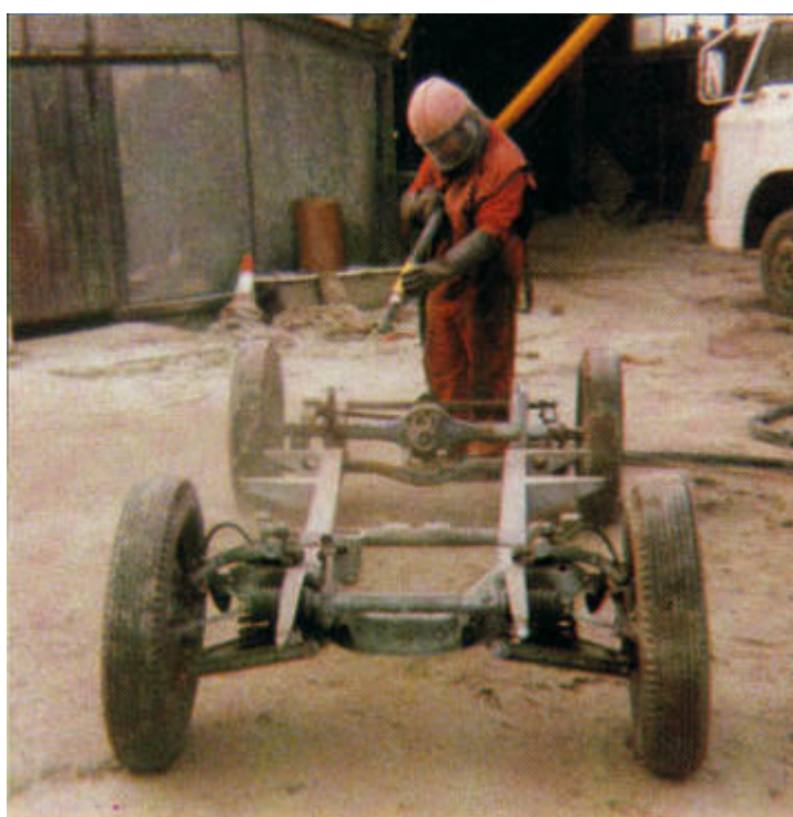
Left and above, despite the condition of the body, the chassis was remarkably good and needed little more than cleaning and painting.
