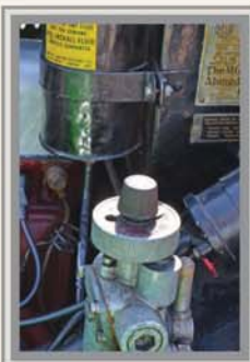
The 'Jack All' system. Select front, back or both, insert the handle, pump then 'up she comes'.
