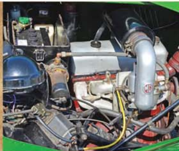
The 1.25-litre engine is reliable and lively, but struggles pulling the nearly one ton Y-Type.
