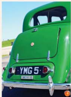
Double doors at the rear include a boot area and a further compartment below for the spare tyre.
