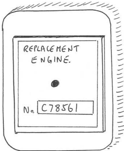
Sketch Five, the later BMC XPAG replacement engine plate, no disc, just a number. "Gold Seal Engine".
