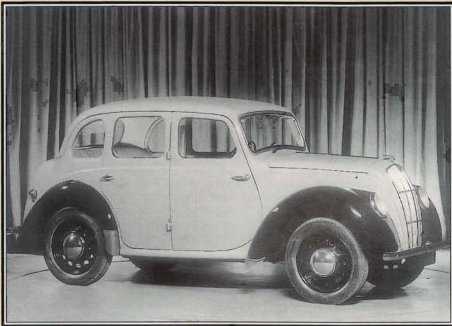
*This picture of a prewar Morris Eight shows clearly the similarity between the body used for that car and the one fitted to the Y-type.*
