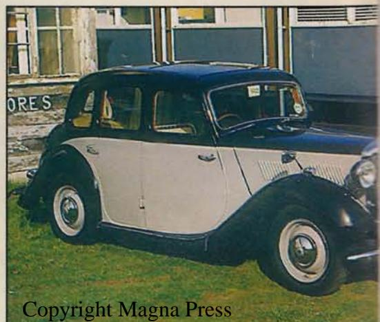
A recent picture of a Y-type painted in a non-original two-tone colour scheme. The factory supplied cars with the body in one colour, the lighter shade, and the wings and running boards in the darker colour.
