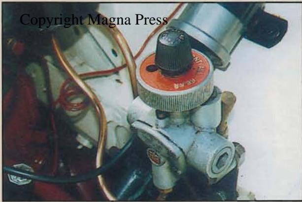
*A useful feature of the Y-type was the 'Jackall' system that allowed you to jack up the car by pumping up hydraulic rams fitted to the front and rear of the car by means of this under-bonnet pump. Either just the front or just the rear, or both ends together, can be raised by choosing the correct position on the selector dial. Twisting the black knob on the top releases pressure and lowers the car.*
