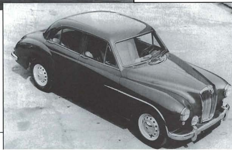
The Wolseley 4/44 used the same basic body as the MG, but sat higher and had swaged-out sills
