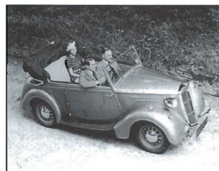
The all-steel Morris Eight Series E body was adapted for the MG
