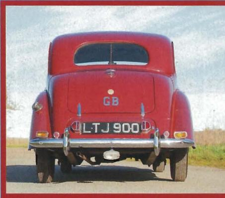
**ABOVE AND RIGHT:** Lighting upgrades include discreet flashing indicators to supplement the trafficators, wired up to operate in tandem from the switch mounted on the steering wheel.
