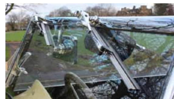
Above: Wipers are mounted along the top of windscreen and use a single motor with an external link.
