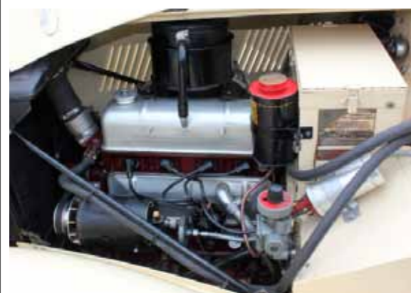
Above: The 54.5bhp/1250cc XPAG engine was considered a lively performer in the 1940s and '50s.
