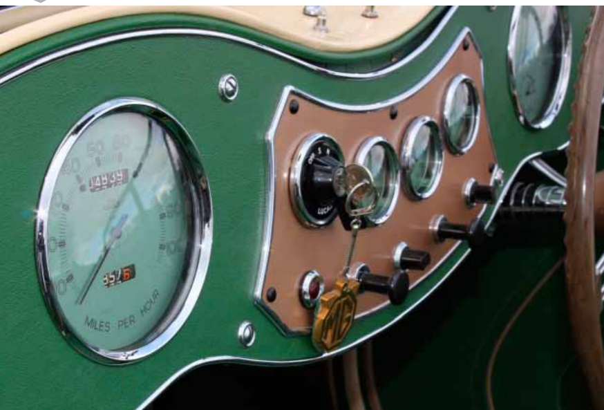
Above: Dashboard has a neat arrangement of Jaeger instruments.
