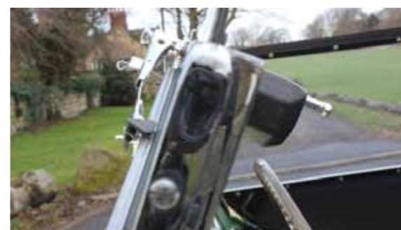
Above: Wipers are mounted along the top of windscreen and use a single motor with an external link.
