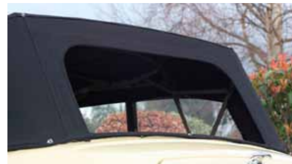
Above: The rear screen can be unzipped and folded down to provide good airflow through the cabin even with the hood up. A neat idea for warmer climates, where the hood can be best used to ward off sunstroke.
