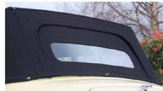
Above: The rear screen can be unzipped and folded down to provide good airflow through the cabin even with the hood up. A neat idea for warmer climates, where the hood can be best used to ward off sunstroke.
