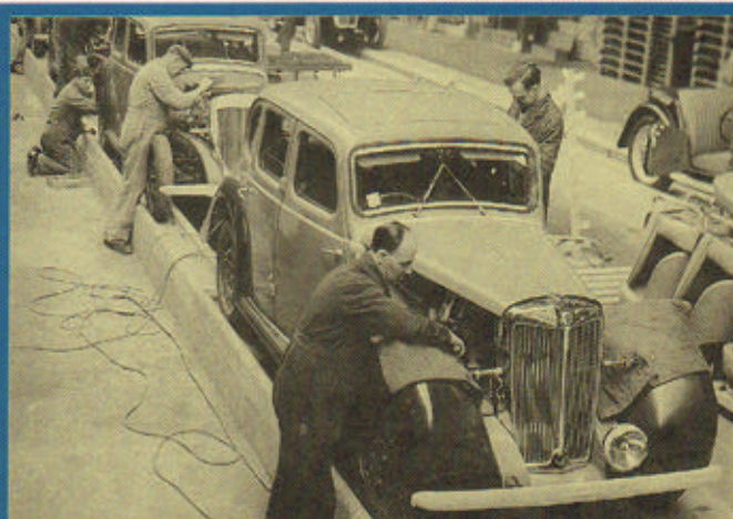
On the "top deck", women workers (above left) installed all the trim and many minor components before the bodies were fitted to the chassis. Above right: Nearing completion, with seats installed and wings fitted, only a few tasks remain to be carried out.
