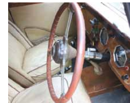
Above: Steering column has telescopic adjustment that combines with seat movement to ensure you get comfy.
