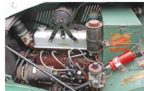
Above: 1250cc XPAG engine was rebuilt in 1998 after the crank sheared, and has done well since.
