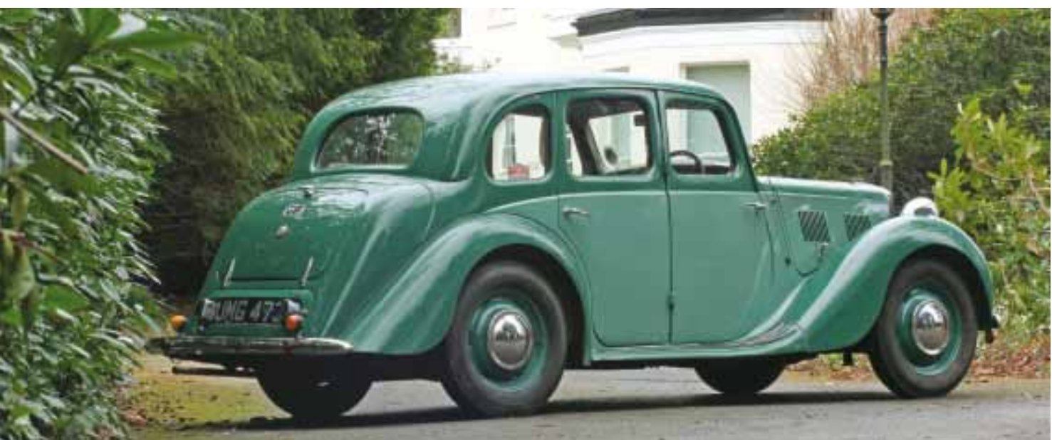
Below : 16in wheels and shallow rear wings mark the YA out from the YB with its 15in wheels.
