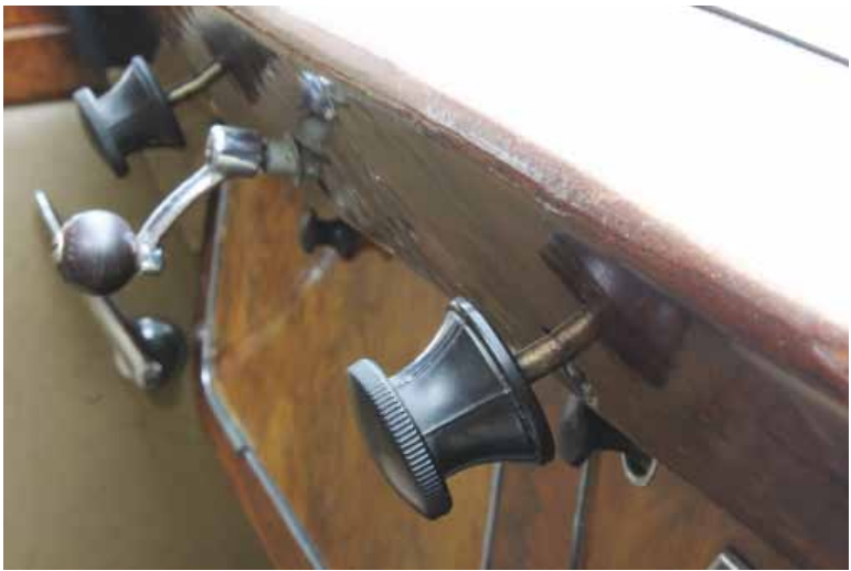
Above: Control knobs allow one or both windscreen wipers to be operated manually or electrically.
