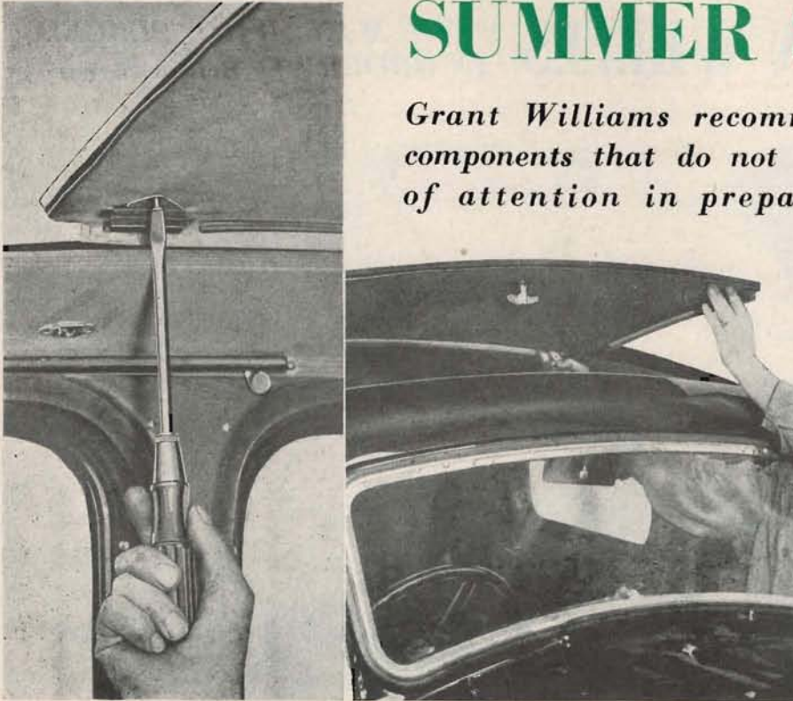
On the left, the retaining screw of one of the sliding roof guide plates, often just hidden by the roof lining cloth, is being slackened before the plate is moved outwards. The roof panel is then drawn forward and lifted out, as shown on the right, complete with the two rear felt guides.
