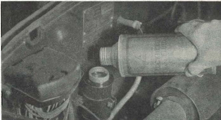
The fluid level in the supply tank should be inspected once a month and replenished if necessary to about one inch below the filler-cap.
