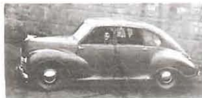
The very first Jowett Javelin prototype. Compare it with a production car — half-frame doors, that grille, and a vee-screen all disappeared on the way.
