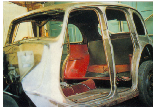
4. Most of the body structure was thankfully sound, but localised repairs were required thanks to a long dead sunroof drain tube.
