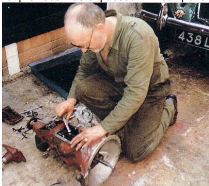
The gearbox was one of YB's few components that needed comprehensive work. Sloppy gear change was cured though.
