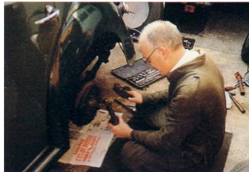
Rear spring hangers were corroded and needed rebuilding
