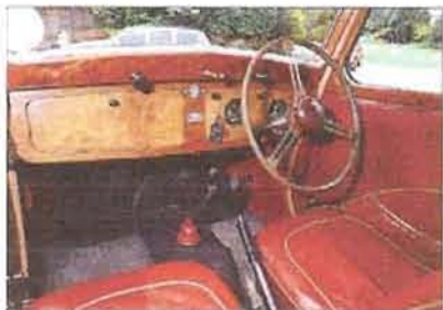
Walnut veneer fascia has been re-varnished
