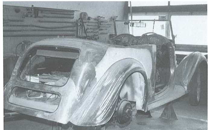
New metal used mainly in the area of the doorsills and rear end.
