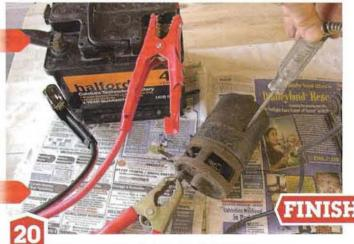
TEST FIELD-COIL FOR EARTH LEAK
