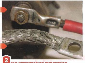
Fractured, frayed or corroded wiring will impede the flow of power and hamper the starter's performance, as will loose, corroded or dirty connections. Check them regularly. Battery terminals and contacts can be weather-proofed with Vaseline or copper grease.
