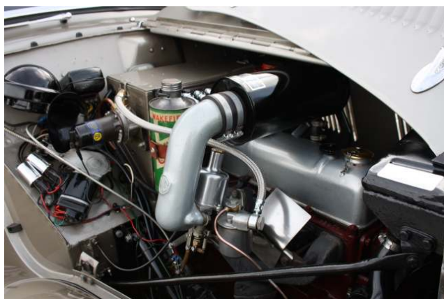
Photo 2 shows the single SU carb set-up in the XPAG of the YA and YB.
