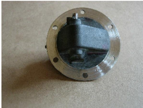
distorted by the chuck or even thrown from the chuck completely. After re-assembling the sender unit it was ready for replacing in the tank. A new gasket and careful tightening of the screws to ensure no distortion and the job is done.
