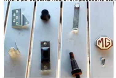
inside a sealed cloth bag. All items were small and unique to Y types and included a boot lid chain attachment plate, a door stop bar rubber, an under front mud guard wiring harness support bracket, the front number plate bracket, rear axle lower bump stop rubber and plate, a bumper bar to chassis pin, a boot chain clip and a boot MG Badge. The author of this article could only identify a couple of them correctly.
