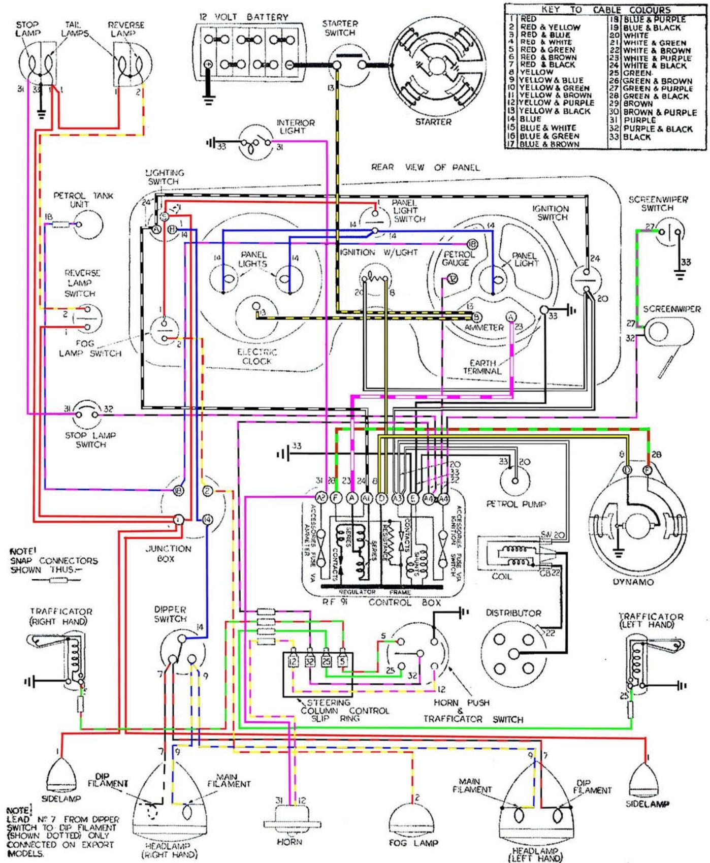
Illustration No. N.26. Diagram of the wiring system, with RF.91 Control Unit.
