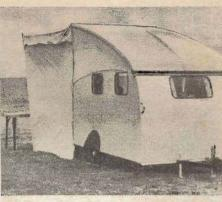
The new Wessex caravan is low built when in travelling trim. When parked, the roof rises on hinges to give head room, and a canopy tent can be added making room for two camp beds.
