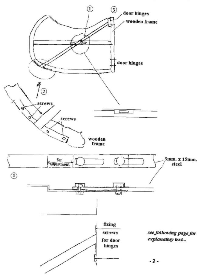
Making an Adjustable Door Cross-brace for the Y/T Door...
