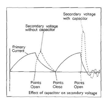
For technophobes, a diagram of what the capacitor actually does by storing power.
