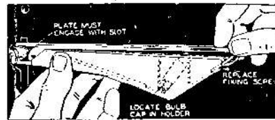
(Above) How to replace the metal strip after fitting new bulb.
