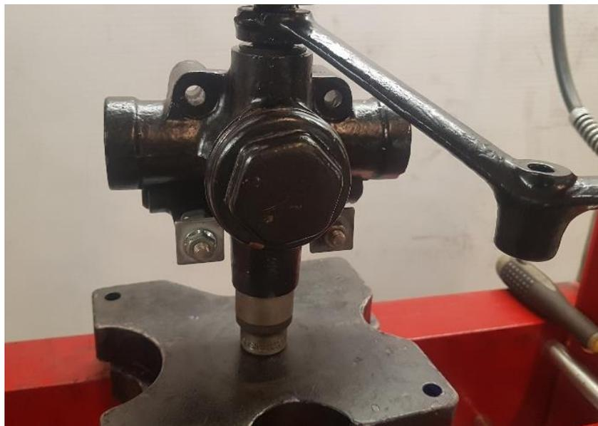
30. Align and press the other *damper arm* onto the axle on the other side. Make sure that the *damper arms* are moving freely. There will be some resistance because of the (old fashion) *rubber seals*.
