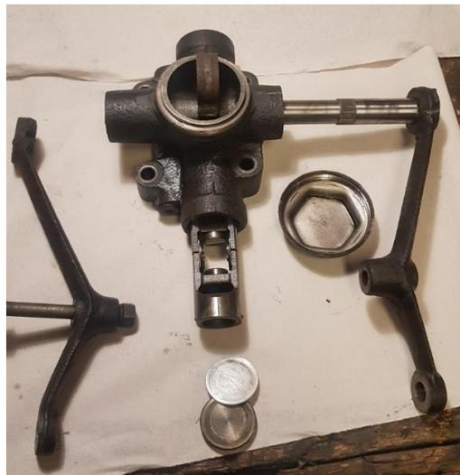
1. Disconnect the *shock absorber* from the front of the car and clean the outside of it.
