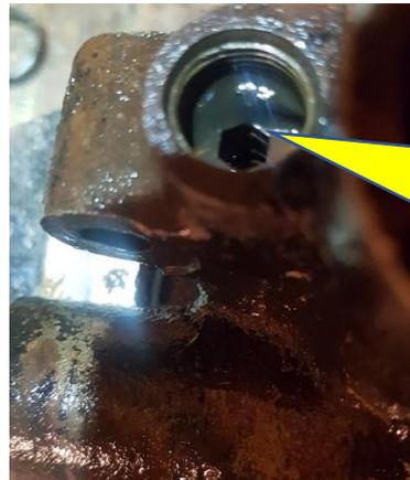
15. Clean out the internal of the *damper housing* and clean all the parts. Scrape/clean away all the remains from the old rubber seals on the housing and the axle shaft. Soak it in solvent, kerosene or diesel. Use a small brush and compressed air to clean out the internal of the damper housing.
