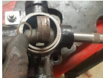
11. The *piston* can now be pushed out of the *damper housing* either way.
