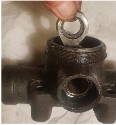
10. Be aware of the washer on the side of the rocker arm that is facing the “small end” of the *damper housing*. This washer is a *thrust washer* for the *axle shaft*, and the *axle shaft* will stop against it when it is pressed back inn to the *damper housing*.
