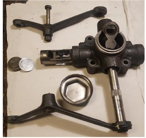
26. Move the *piston* to its end position towards the direction of the *Damper arms*.
