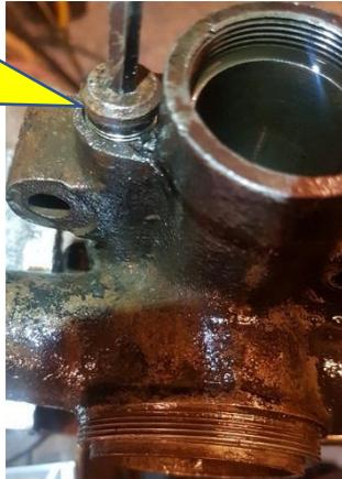
The Valve Adjusting Screw under the plug.
