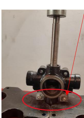
8. Press out the *axle shaft*. See that the *damper arm* under is not hooked up in anything while pressing the *axle* and *damper arm* down.
