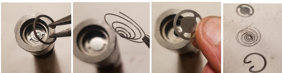
13. Assembly the valve with the center top of the spring facing down against the aluminum disk. See that the “lose end” on the big diameter of the spring is not hooking in to or getting caught in the groove for the circlip when the circlip is put back.
