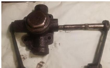
9. Take the *rocker arm* out up through the filler hole. It can be a bit tricky to get it out because its fitment down into the *piston* is slightly spring loaded, and the clearance against the internal sides of the *damper housing* is tight.
