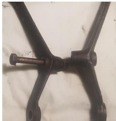
4. Pull off the "small end" arm with a pulley. (It will also come off when the *axle* is pressed out through it.) The other arm is fixed to the "big end" of the *axle* with a spline and is coming off together with the *axle*.
