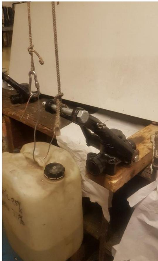
39. Adjust the damper force (time of the movement for a full stroke from top to bottom or bottom to top) with the two *Valve Adjustment Screws*. See #14.
