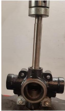
17. Make a suitable tool/drive pin for driving out and putting back the two *bearing bushes*.
