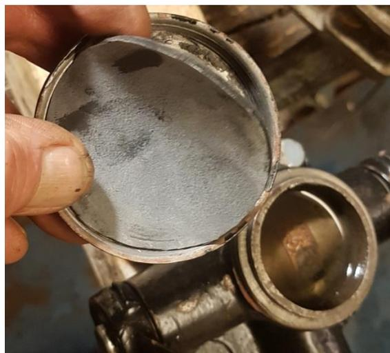
32. Fill up the *damper housing* with hydraulic oil ISO 32, or any motorcycle front fork damper oil. It is important to write down and use the same type (viscosity) of oil when/if refilling. Because the damper setting (next chapter) is based on that type of oil.
