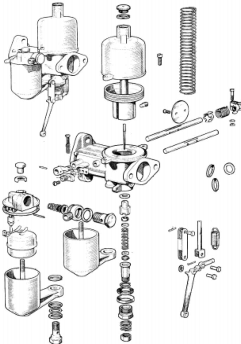
**S.U. H4 1 1/2 inch AUC 818 Carburettor used on Mini or Sprite Shorrock C75B Superchargers**
