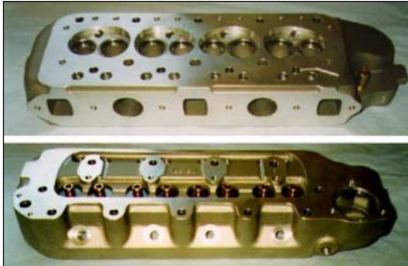
NEW ALLOY HEAD WITH 23CC CHAMBER WITH 30% IMPROVEMENT IN POWER WITH EXCELLENT COOLING PROPERTIES FOR SUPERCHARGING. A BOLT ON MOD FOR 1275CC ENGINES. YOU WILL HAVE TO POCKET A BLOCK IF USED ON 850.948, 977, 998 AND 1098CC ENGINES.
