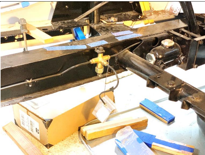
4-Way. Dangling line not connected to M/C
