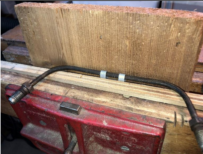
Step 3: Squeeze top of strap between two loose pieces of wood to start rounding the strap
