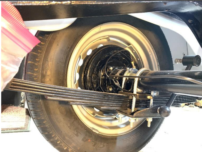
Left rear. Bend at check strap and wheel cyl. Line goes around check straps – not through . (The check strap is not mounted.)
