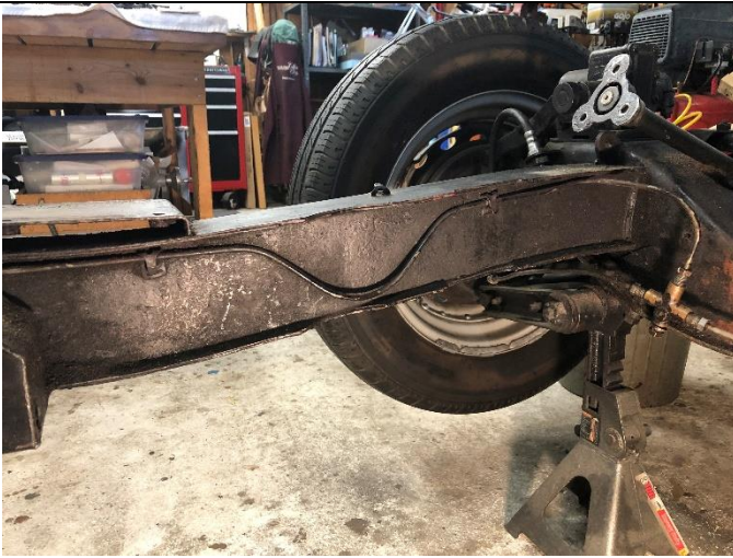
Left Front. 3-Way. Routing and attachment to wheel cylinder similar to right front. Note "V" in this original 46-inch brake line, TF7211.
