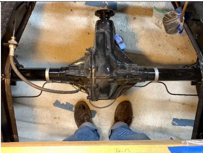
Diff top view. Note bends and straps. Lines should be tighter to pumpkin.
