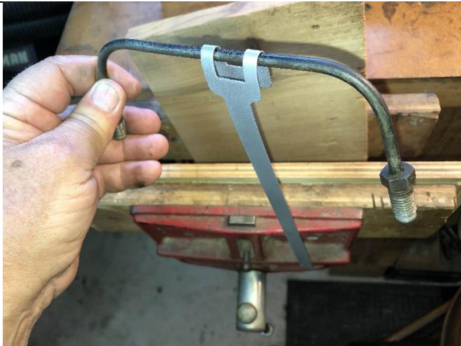
Step 1: Bend open end over a piece of old brake line as shown.
