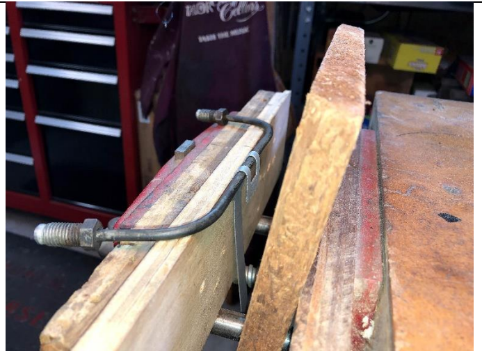
Step 2: Set strap and old brake line in vice with loose faces as shown.
