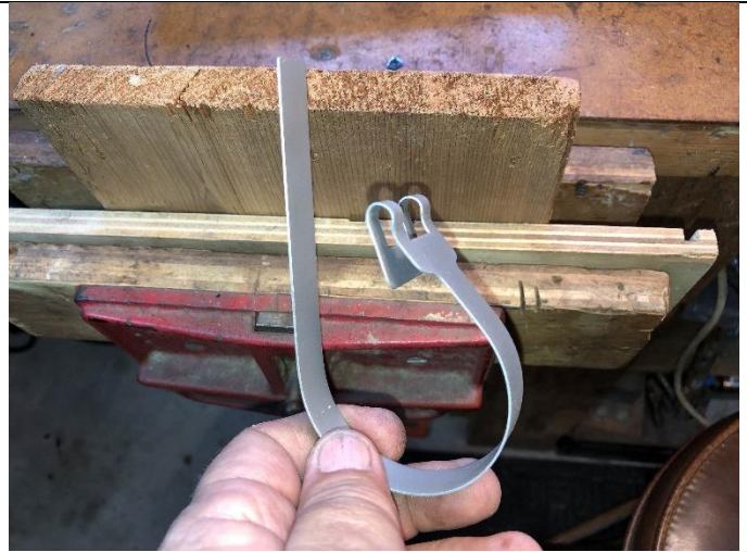
Step 4 – Pre-bend the strap for the axle tubes.
