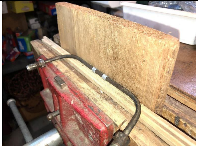
Step 3 continued: See how open end of strap bends over the loose wood nearest to the Tommy bar.
