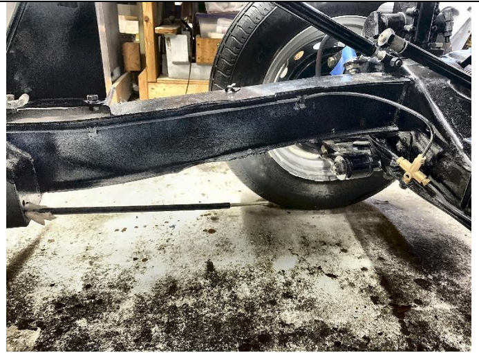
Left Front. 3-Way. New 43-inch line, TF7211. Line is straight. I did not have enough line to bend the "V". See original "V" in photo at left.
