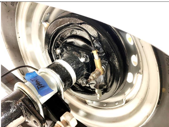
Left Rear. Front view – YIKES Brake line is not connected to wheel cylinder!
