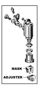
**DETAILS.** Use 1/8" steel bar stock or 1/8" thick angle bracket purchased from a hardware store or use something similar lying around the shop. Cut the shim 1-1/8" long X 1/2" (or 9/16") wide. Tack weld the ends of the shims to the adjuster masks. Do not weld the sides. After welding, file the top flat and remove weld material on the underside of the mask that may interfere with the adjuster. If you can't weld, then a club member can probably do the job for you. SafetyFast!
