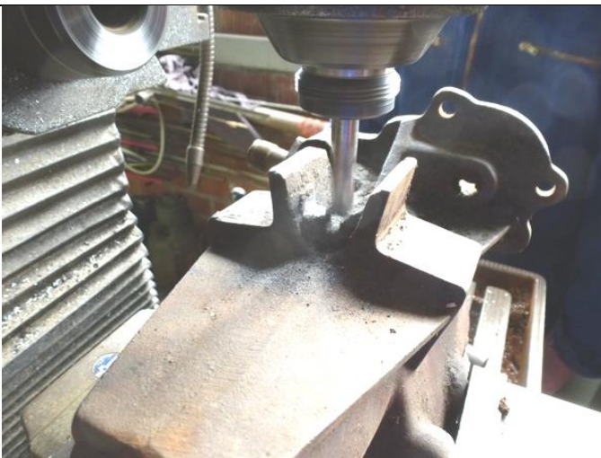
Milling the web – removing the broken eye
