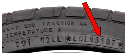
The date code is usually on only one side of the tire, so you may need to crawl under the car to read it
