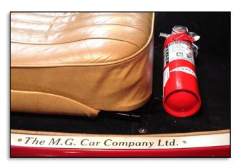
Note: New Halon extinguishers are no longer available because it depletes the ozone. Less effective, ozone friendly Halotron replaced Halon. Halon from old extinguishers can be reclaimed and used.
