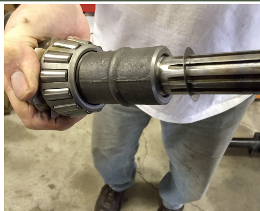
Pinion prior to spacer & bearing removal.
