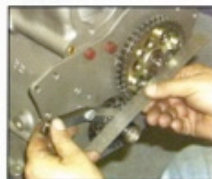
If these gears run out of line that's not good for chain life, or the gears!
