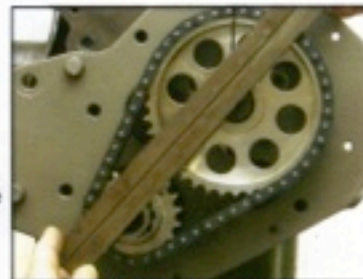
The straight edge line should go through the cam/crank shaft centers as well as the two gear 'dots'.
