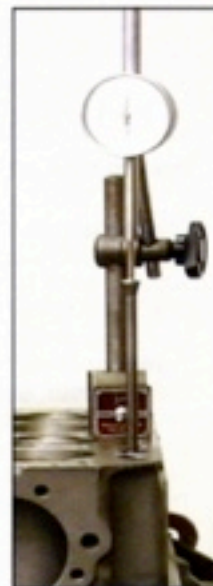
Reading lift on cylinder #1 inlet lobe. Remember this is normally the second hole from the front.
