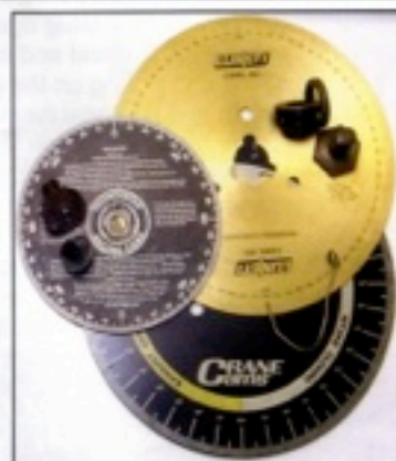
These are the degree wheels we use in the APT shop. The Lunati wheel has a separate lockable hub a Mini flywheel bolt holds it to the crank on BMC engines
