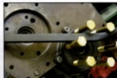
Turn the crank like this. Do NOT use your new ARP flywheel bolts for this
