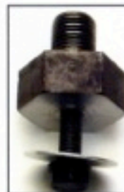
This crank bolt has a register on the front face to locate the degree wheel
