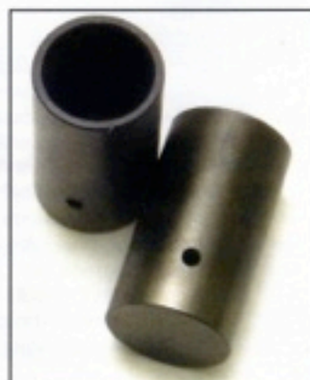
APT manufacturers their own special chilled iron cam follower for BMC 'A' & 'B' series engines. Part number CF-04 Also available for Triumph 1147—1500, GT6, TR6 Part number CF-10 4 cylinder Part number CF-11 6 cylinder These have the oil drain hole. Face hardness is Rc63 and is manganese phosphate coated for easy break in when used with cam lube and ZDDP in the oil.
