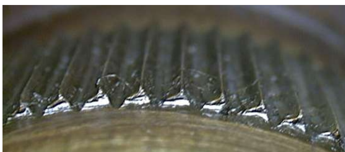
Bad: Hub spline very badly worn - skewed flank and sharp apex.
