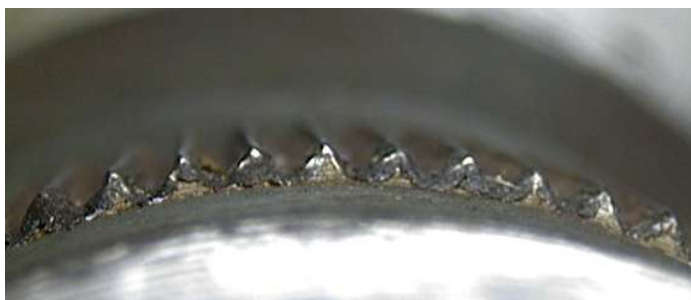
Better: Hub spline moderately worn - but still rounded on the apex.
