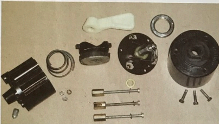
These parts are found in the Lucas vacuum switch of the style without a U-shaped contact.
