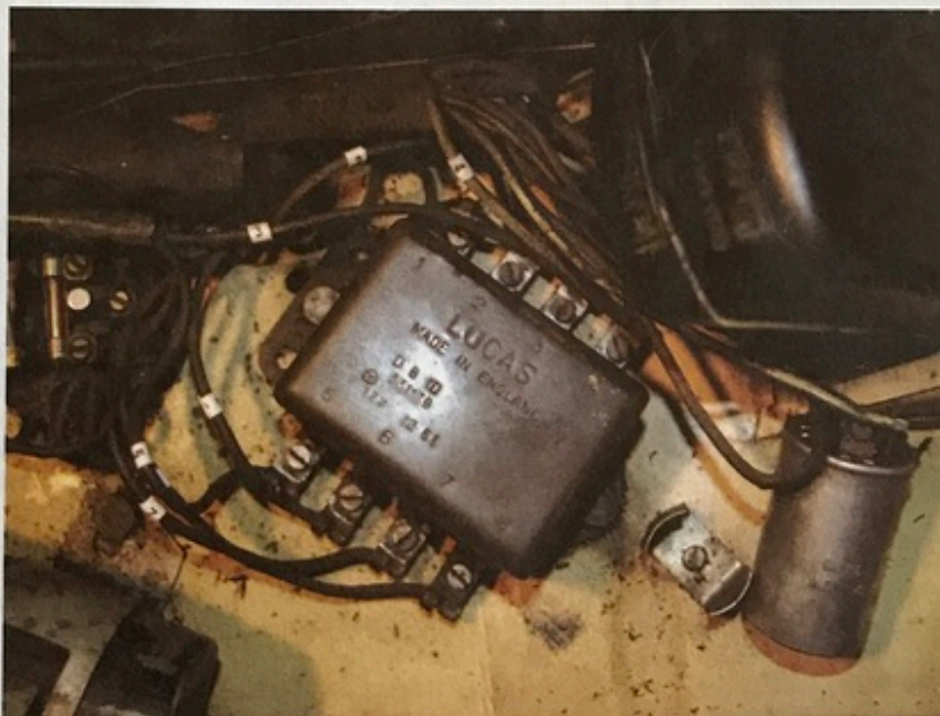
Though the Lucas switch did not function properly, it was not the reason that the blinkers and brake lights stopped working. The problem was in this Lucas relay mounted on the firewall.
