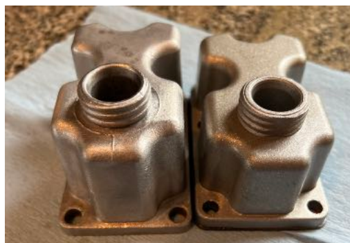
The one on the right is correct the one on the left is aftermarket. The size difference is substantial enough to install it but it will be standing proud of the cowl.
