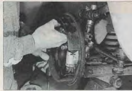
3 The brake backplate can be lifted off after undoing four bolts. It is a good idea to protect brake linings from oily hands with masking tape.
