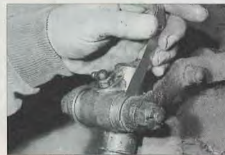
9 There must be .008in. - .013in. clearance between the trunnions and thrust washers when fulcrum bolt is fully tightened. Seals omitted for clarity.
