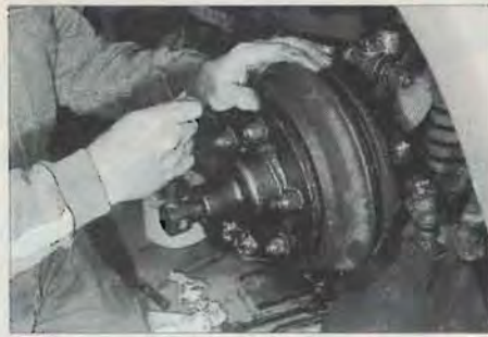
2 Using a puller to remove the hub; don't forget to slacken the adjusters first and to uncouple the brake hose and steering tie rod.
